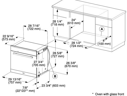
Cut-out (4" x 28" / 100 mm x 720 mm) in the bottom of the cabinet for power  $(\mathbf{A})$ cord and ventilation
